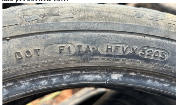
Figure 1: Example of a DOT number. F1 indicates the Manufacturer as Michelin Tyre PLC in Dundee, Scotland, the last digits explain the manufacturing date. Here 32 refers to week 32 and 05 refers to the year 2005. This means that this tyre was produced between August 08 th - 14 th in Dundee, Scotland by Michelin Tyre PLC.
