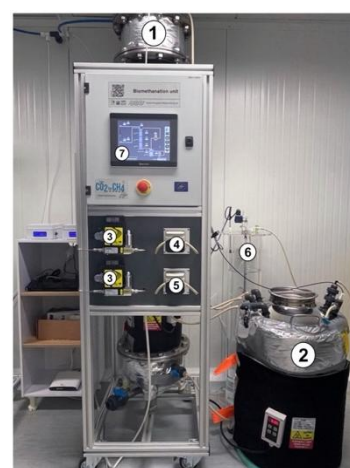
Figure 1. Photo of the prototype pilot methanation unit; (1) pilot reactor, (2) nutrient sump, (3) gases mass flow controllers, (4) nutrient recirculation pump, (5) nutrient sump mixing pump, (6) water displacement gas-metering system.
