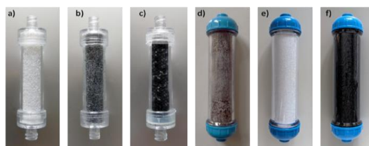
Figure 1. Cartridge filled with granules: a-c: prototypes, d-f standard sized cartridges. a) PSU (0.4 g), b) PSU-GO (0.73 g), c) GAC (2.3 g), d) PSU-GO granules (33 g), e) PSU granules (33 g), f) GAC (130 g).
