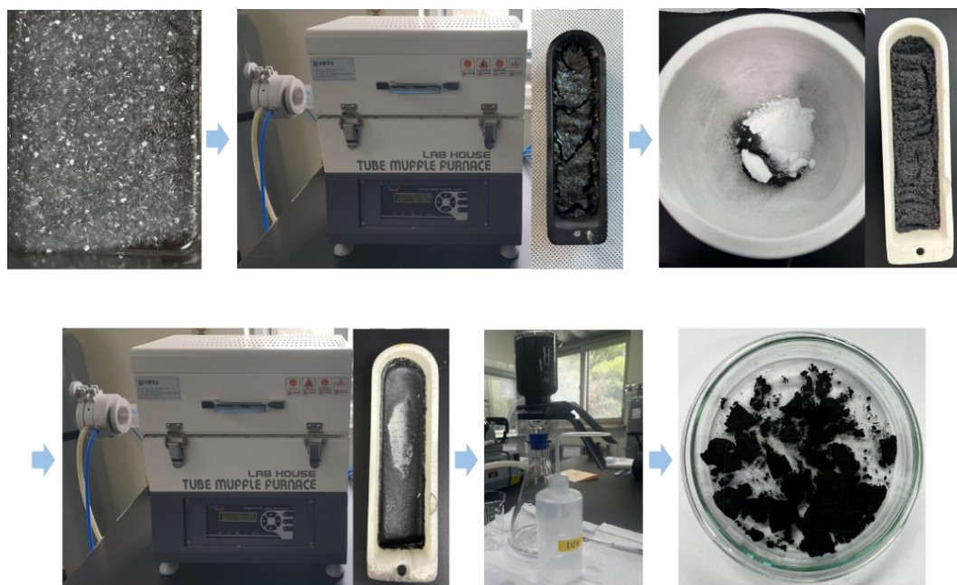
Figure 1. Preparation procedure of N-doped mesoporous carbon catalyst derived from waste PET
