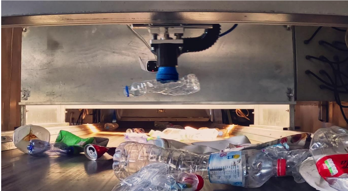
Figure2. AI-powered robotic material recovery inside the prMRF.
